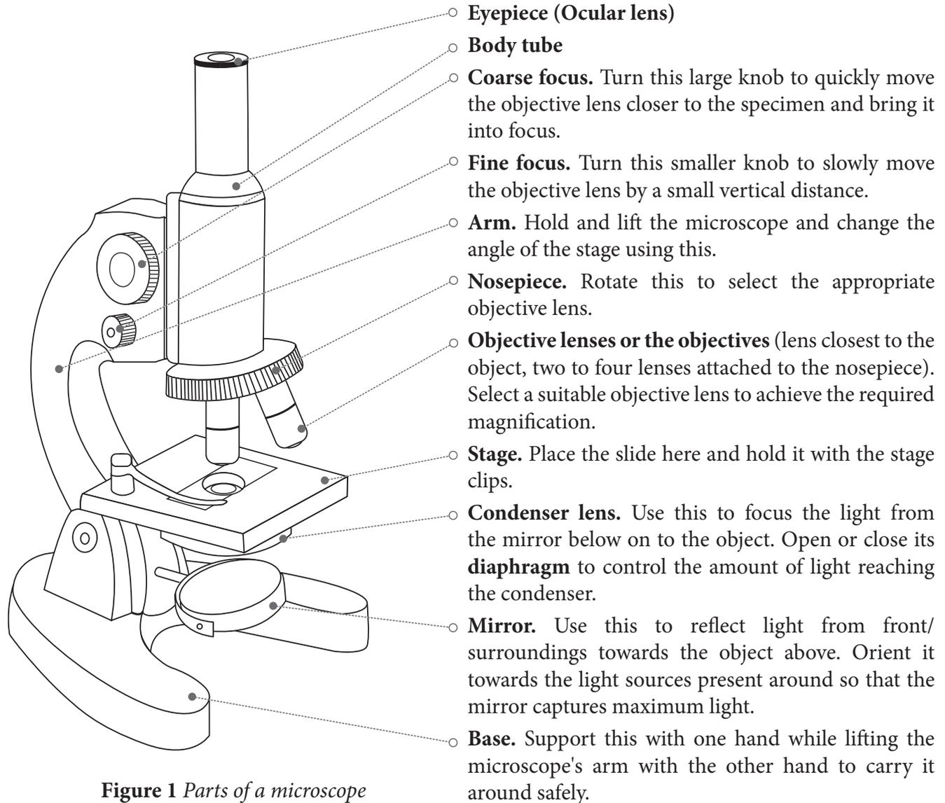
**Figure 1** Parts of a microscope
