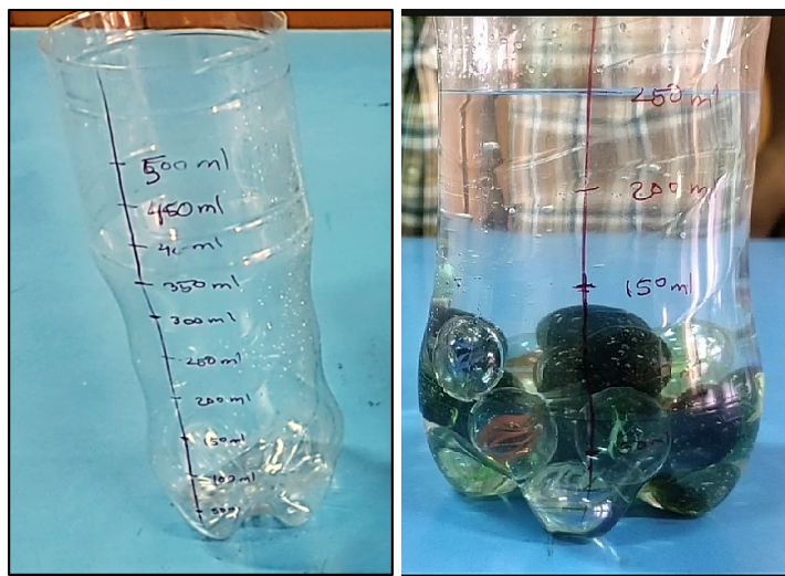
Figure T1: (Left) A measuring cylinder and (right) A measuring cylinder with water and marbles
