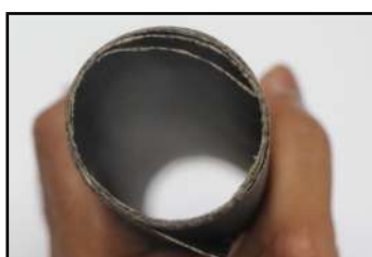
Fig. 2(b): Cardpaper as pipe
